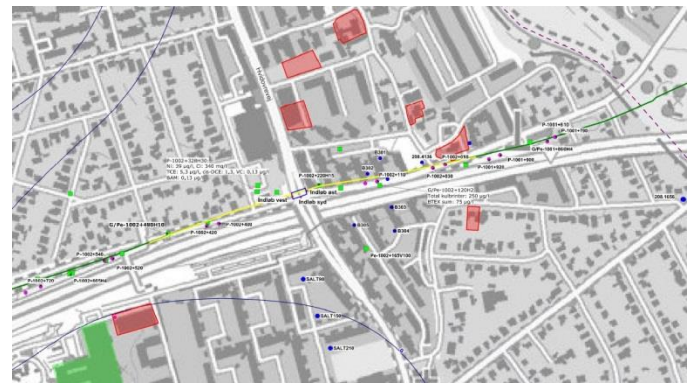
Figure 2 Location plan showing Hvidovre Tunnel and troughs, investigation boreholes and contaminated sites in Hvidovre Municipality.
